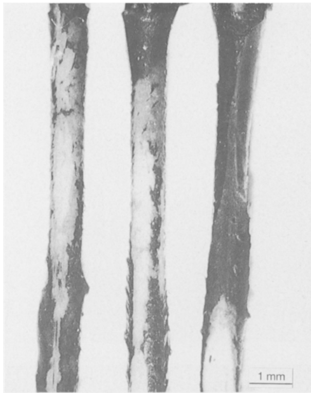
Figure 3 Optical micrograph of the pull-out region of sample B, modified with resorcinol including RF.
