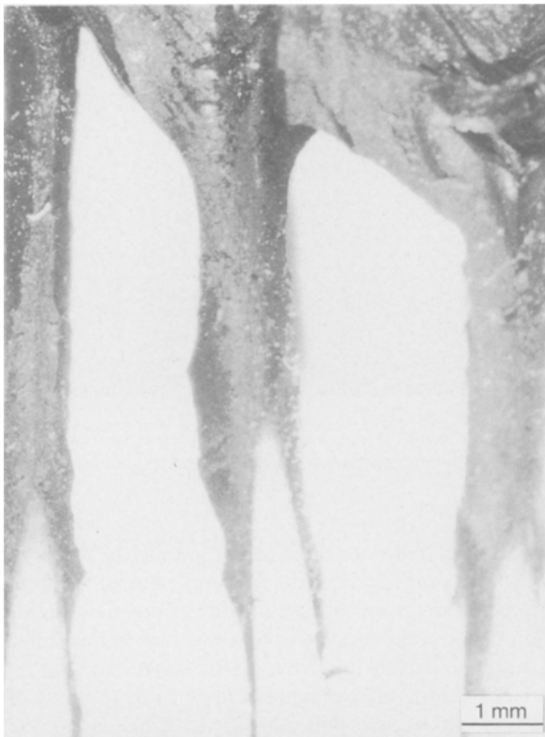
Figure 4 Optical micrograph of the pull-out region of sample C, modified with resorcinol including RFL.
